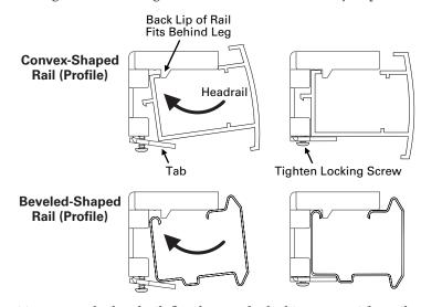
To remove the headrail, first loosen the locking screw. Then tilt the headrail back and slide it out of the installation brackets.
