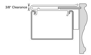
To gain this clearance, use the bracket spacers included with your order (one for each installation bracket and two for each support bracket).
